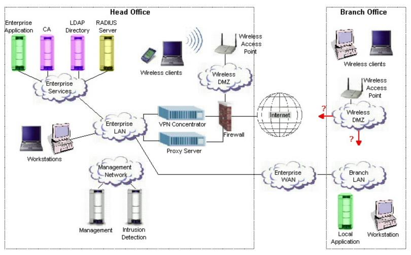
Source: Based on diagrams developed by Andre Carrington for Center for Internet Security Wireless Benchmark using DoD graphics
